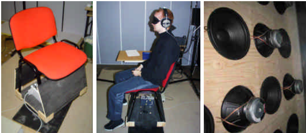
Figure 1: Left: Experimental chair mounted on a turntable to suggest to participants that they could potentially be rotating physically (which never happened during the experiment). Middle: Participant fitted with headphones and blindfold (right). Four fake loudspeakers were mounted on the walls to suggest that the sound presented via headphones might in fact be originating from the stationary loudspeakers. One of the fake loudspeakers can be seen in the upper right corner of the picture. Right: Subwoofer array used for the subsonic stimulation.
