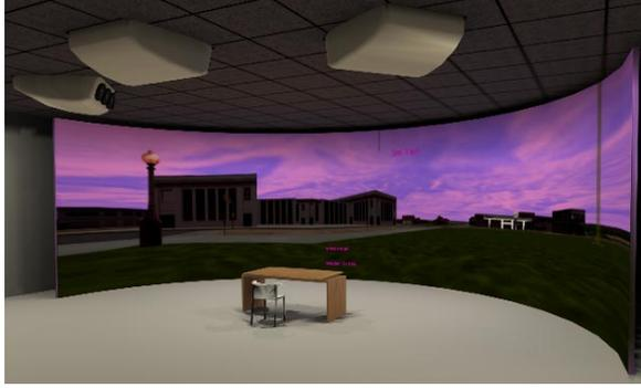
Figure 1: Virtual environment lab with 180° projection screen displaying the town environment. The subject is seated behind the table in the center of the half-cylindric screen. On the table are mouse and keyboard as input devices.
